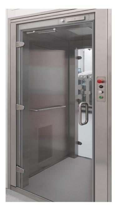
The PBSC fogging shower is a floor mouned personnel shower to be used either on a routine operational basis or in emergencies. The fogging shower fine fog automated cycle is used for the encapsulation of Powders (typically APIs) usually on disposable operatives suits.
